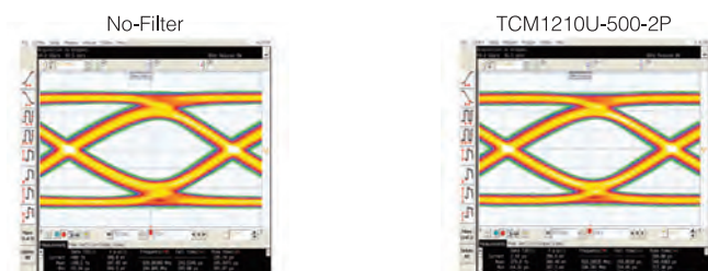
(c) DisplayPort waveform at receiving baseplate using 10m cable (2.7 Gbps during transmission)
