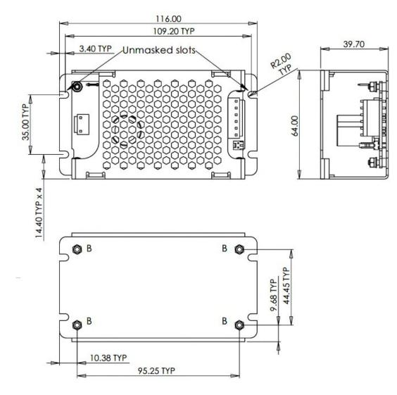
NOTE: B - 4 OFF M3 FIXING - max thread penetration 4.25 mm RECOMMENDED TORQUE - M3 - 0.5 - 0.6 Nm
