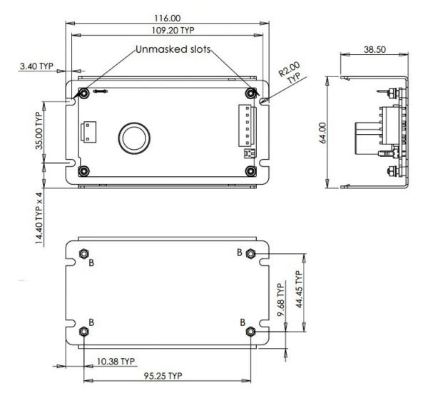
NOTE: B - 4 OFF M3 FIXING - max thread penetration 4.25 mm RECOMMENDED TORQUE - M3 - 0.5 - 0.6 Nm
