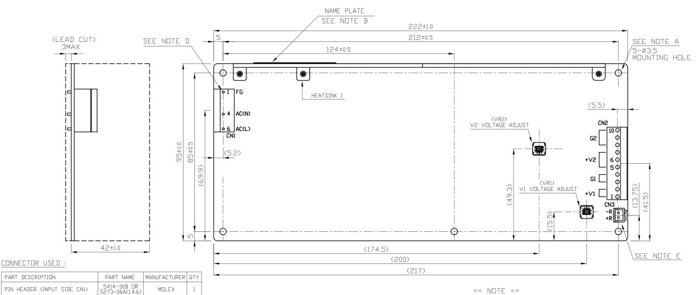
\* CURRENT OF THE CN2 CONNECTOR PIN MUST BE LESS THAN 5A (7A AT PEAK LOAD)
