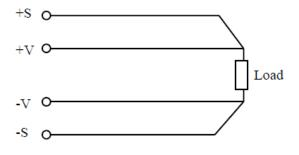
Ensure that the remote sense cables are twisted pairs.
