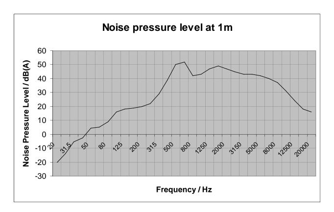
The quiet fan option is typically 5dB(A) lower than the standard airflow version. Reverse airflow configurations are typically 5dB(A) higher then the standard airflow version.
