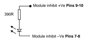
Internal to the module inhibit/enable is a 390ohm 1/8W resistor and the diode of an opto-coupler.
