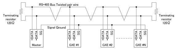
Be sure to connect the data line [+ DATA / - DATA] with a twisted pair wire.
