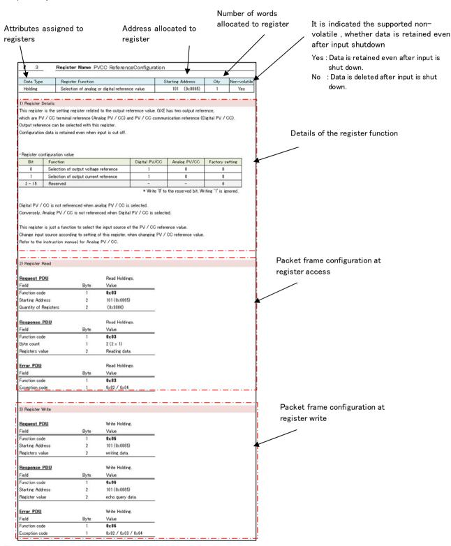
The packet frame described on each page is an example of access to one register.
