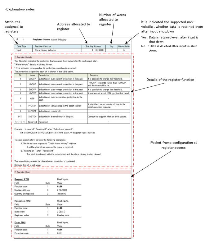
The packet frame described on each page is an example of access to one register. Multiple access is possible when the register address assignment is continuous.
