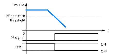
In order to prevent signal fluttering, it is possible to set the confirmation time limit by setting the [PF count] register.
