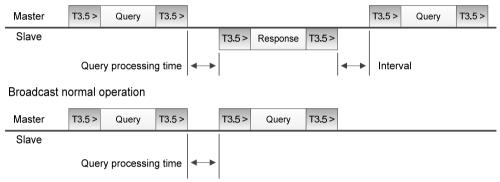
"Turn around time" is the time the master device must waits to complete the query processing of the slave device when issuing the broadcast query. It is normally specified by the communication specification of the slave device. Set the communication timeout of the master device to 100ms or more in consideration of the query processing time of the slave device.
