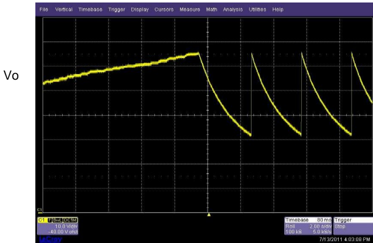
Output Voltage during OVP mode (0% Load)
