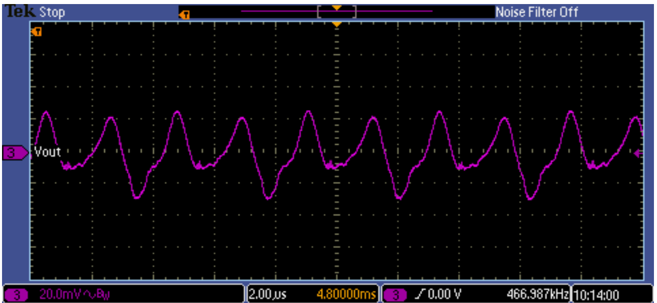
Vout: 20mV/div 2us/div Output Ripple (100% Load, 220VAC input)
