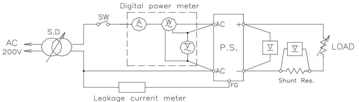
NOTE : Leakage current measured through a 1k ohm resistor.
