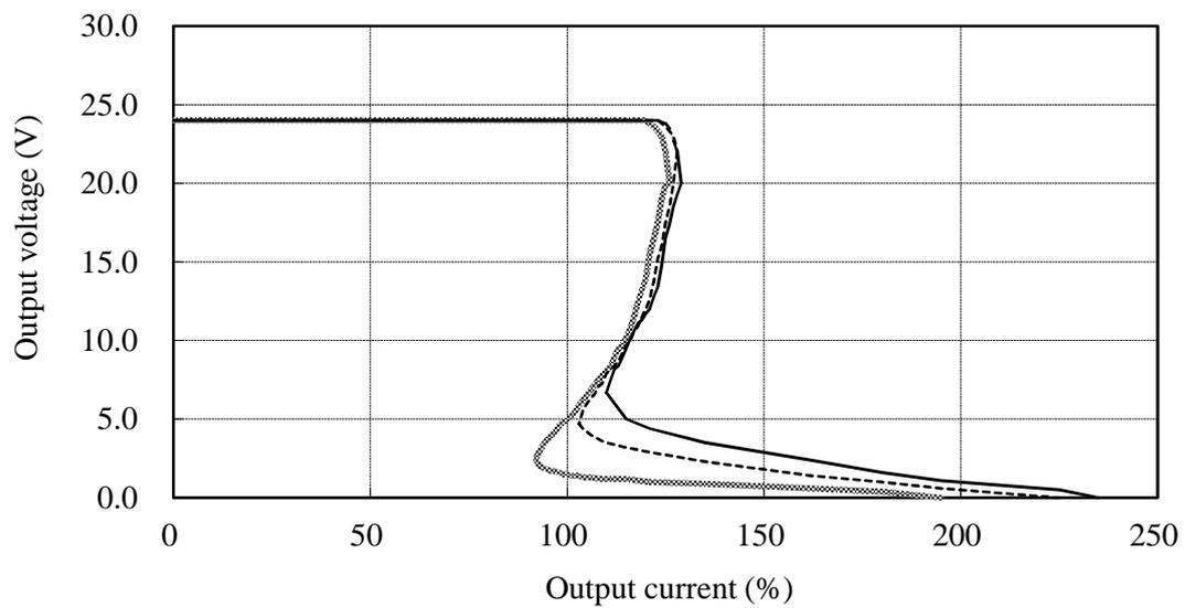
2.4 Over voltage protection (OVP) characteristics
