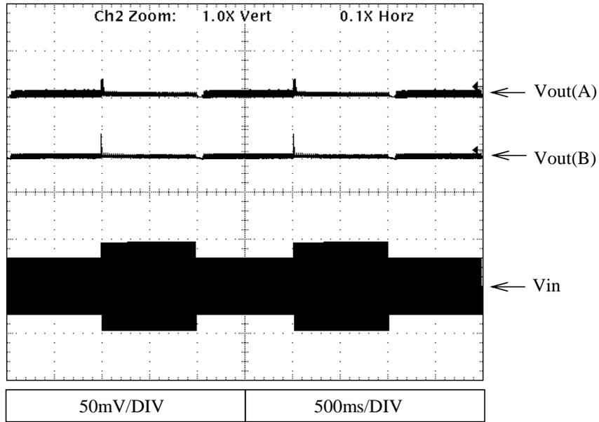
2.8 Input voltage DIP test
