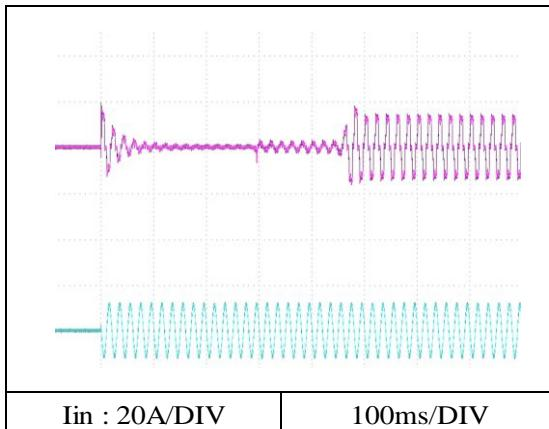
Switch on phase angle of input AC voltage
