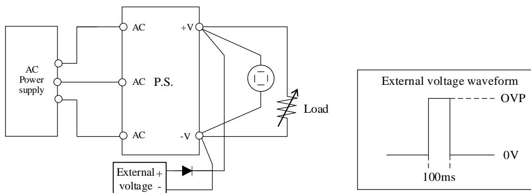
**測定回路 4 Circuit 4 used for determination**
