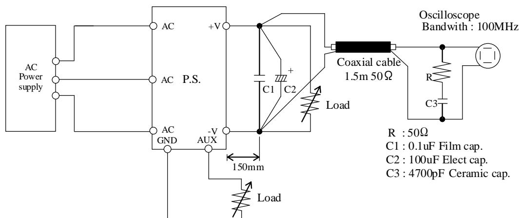
測定構成 Configuration used for determination
