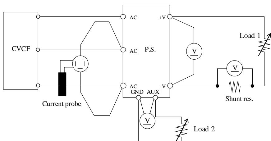
**測定回路 5 Circuit 5 used for determination**
