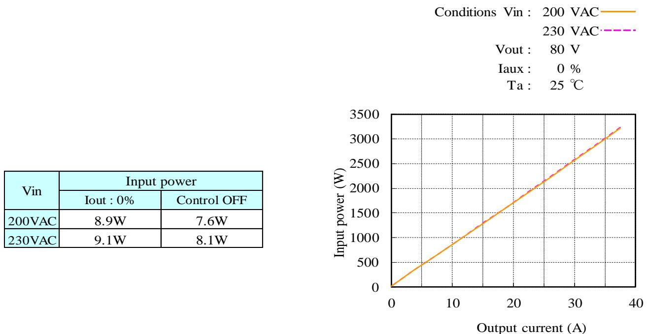
**(5) 入力電流対出力電流 Input current vs. Output current**
