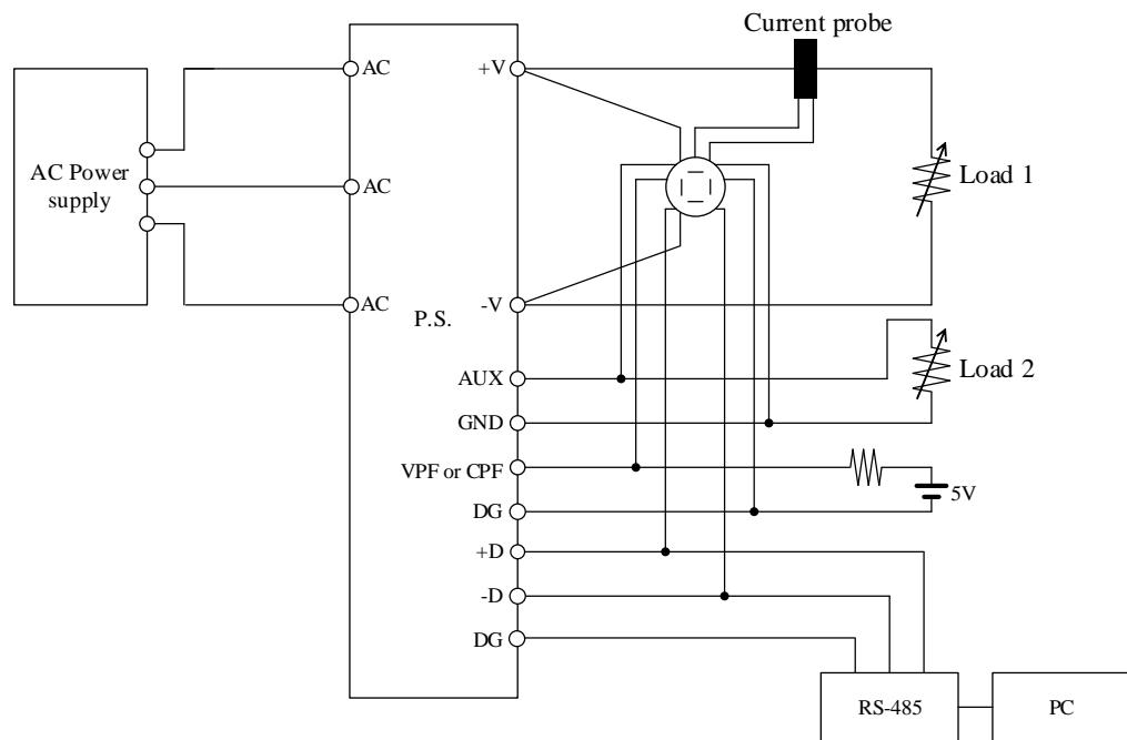
測定回路 6 Circuit 6 used for determination
