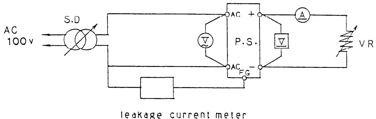
leakage current meter
