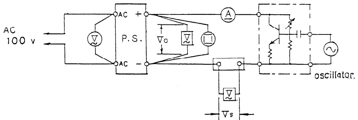
Note : Output impedance  $| Z | = \frac{V_s}{I} \cdot R_s$  ( $R_s: 0.1\Omega$ )
