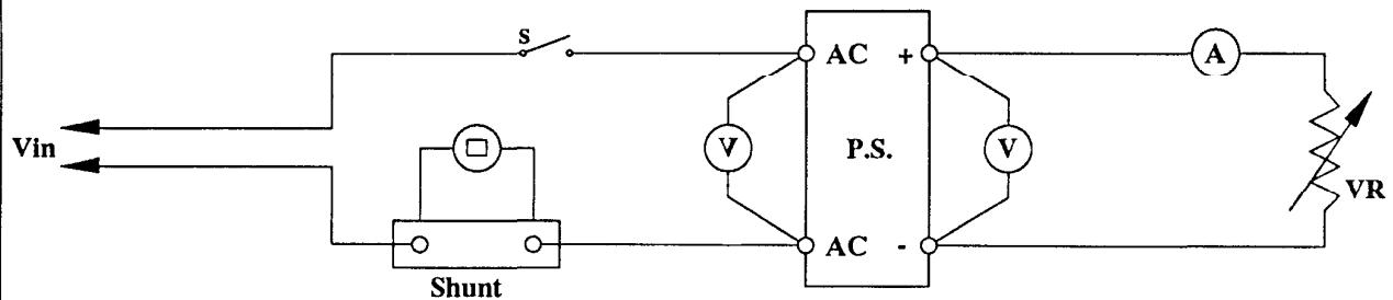
(10) Leakage current characteristics
