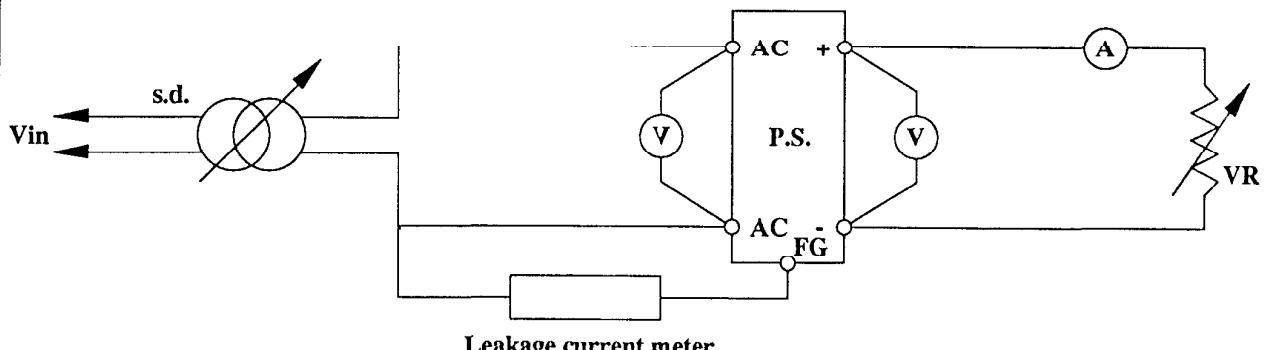
Leakage current meter
