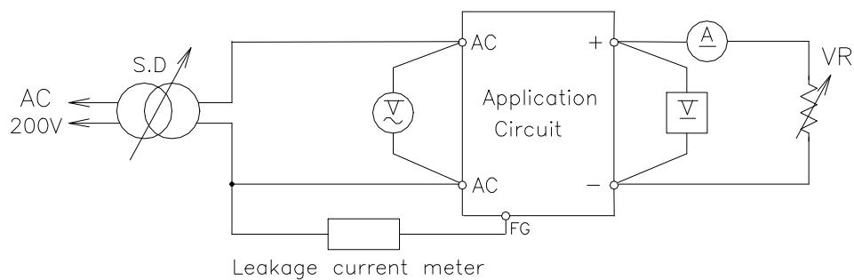
NOTE : Leakage current measured through a 1k ohm resistor.
