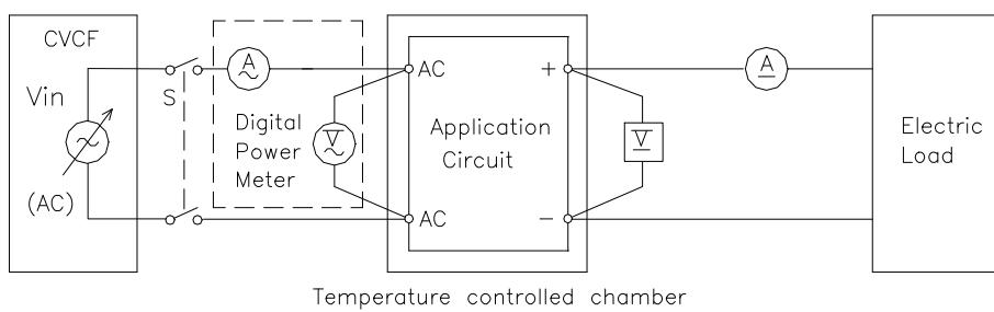
(3) 電流制限特性 Current limit characteristics
