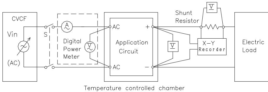
(4) 過電圧保護特性 Over voltage protection (O.V.P.) characteristics
