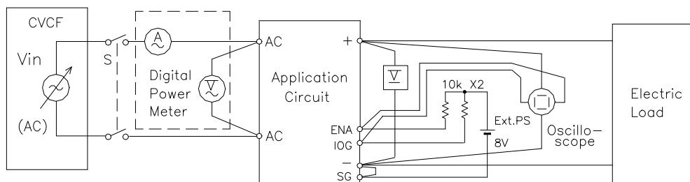
(8) 過渡応答（入力急変）特性 Dynamic line response characteristics
