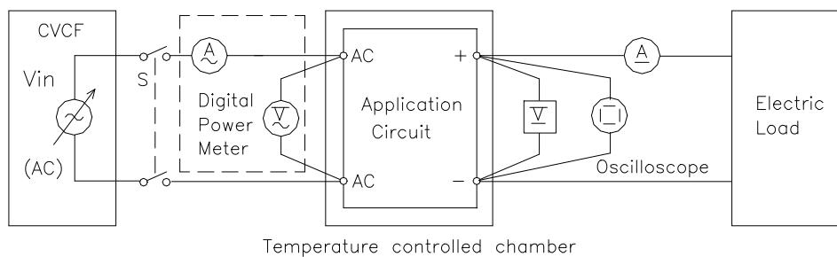
(2) 通電ドリフト特性 Warm up voltage drift characteristics
