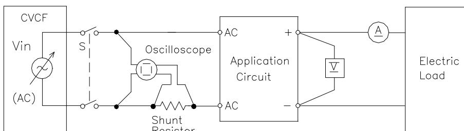
(11) 入力電流波形 Input current waveform
