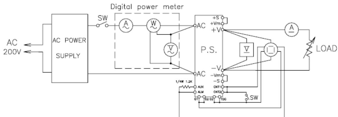
(8) Output fall characteristics with ON/OFF CONTROL
