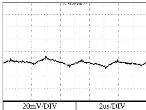
**2-18 Output ripple and noise waveform**
