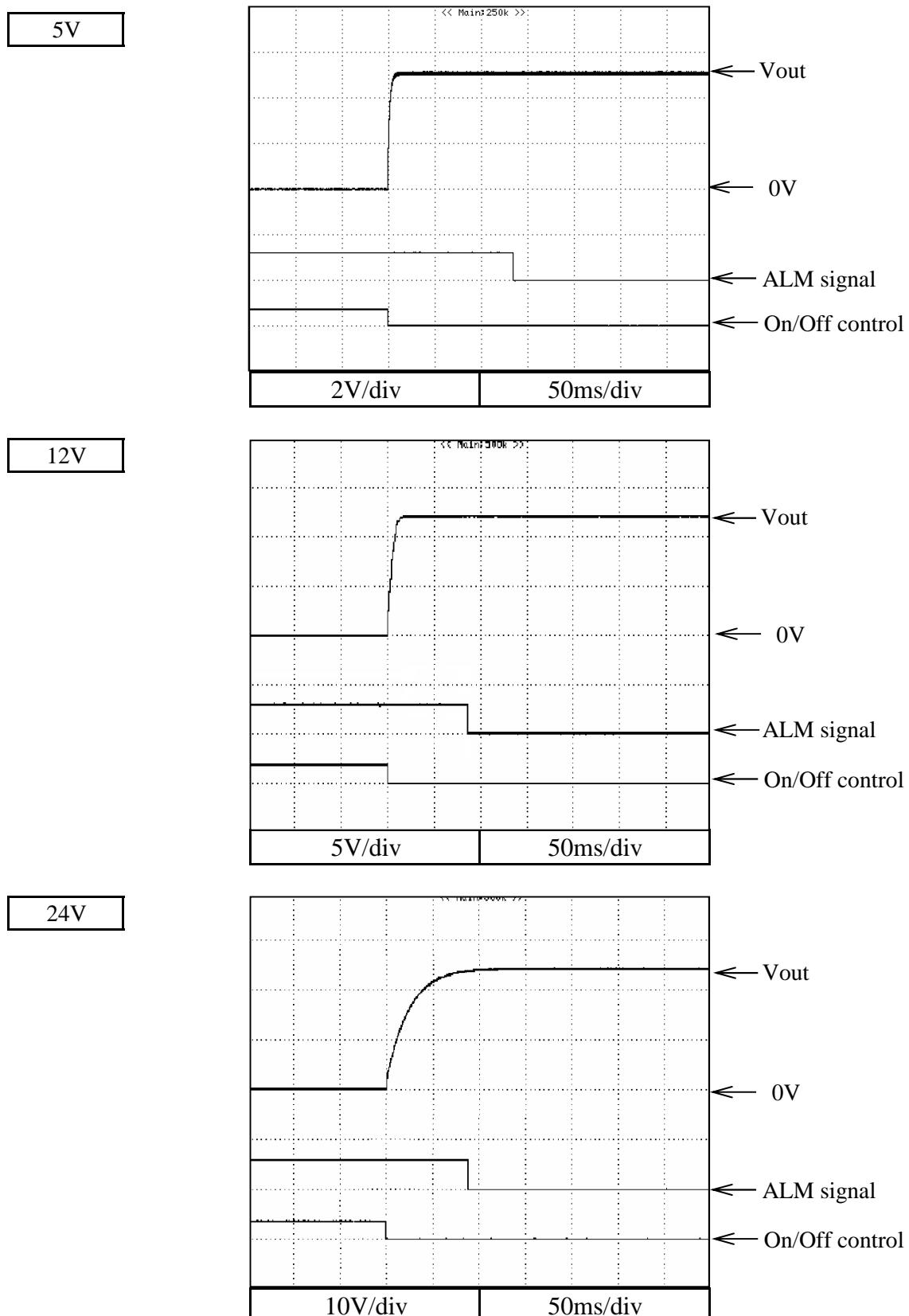
**2.8 Output fall characteristics with On/Off control**
