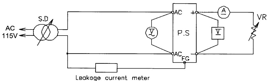
Note :    Leakage current measured through a 1k ohm resistor.
