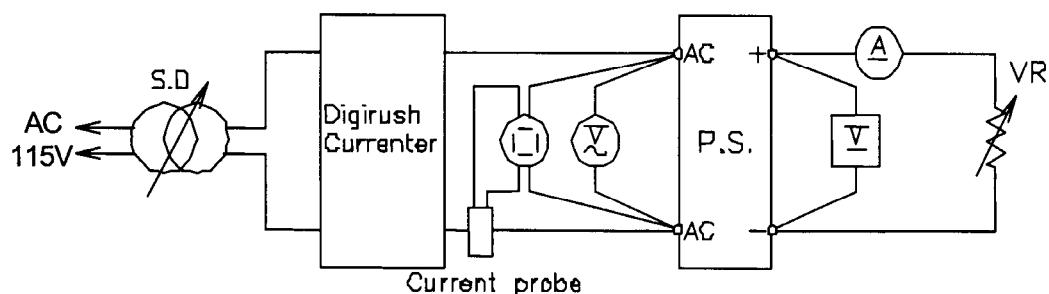
(8) Leakage current characteristics
