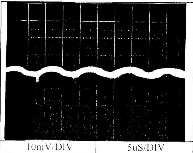
2.14 Output ripple and noise waveform
