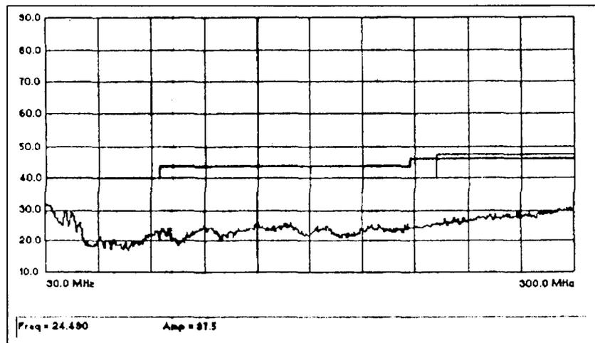
2.15 Electro Magnetic Interference characteristics
