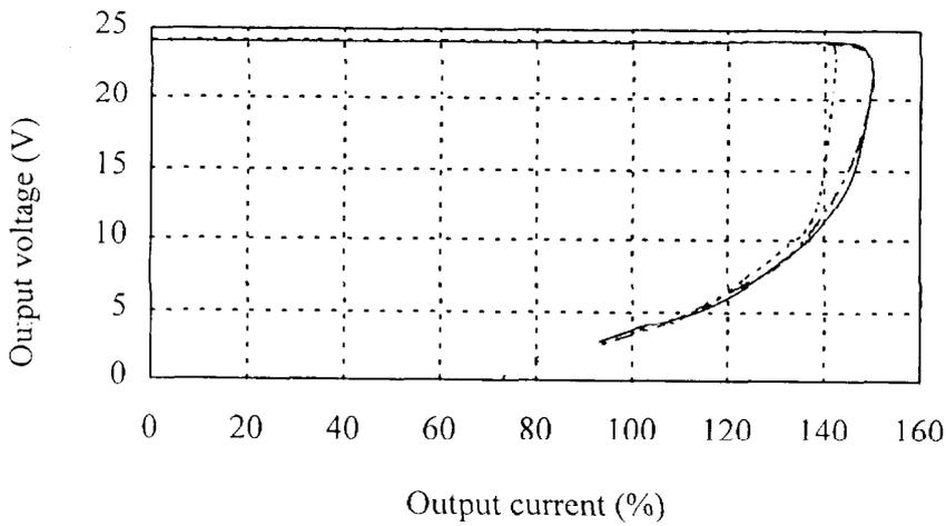
2.4 Over voltage protection (OVP) characteristics
