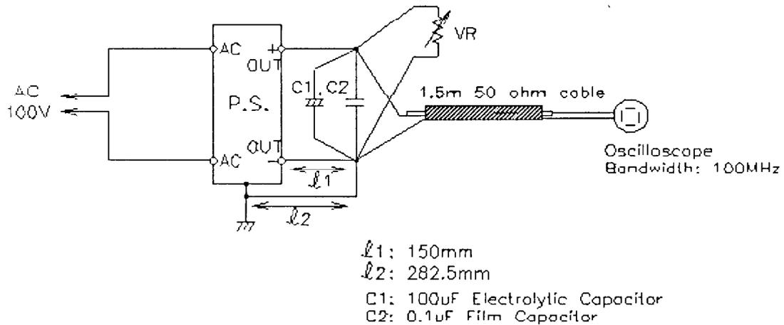
12) Electro-Magnetic Interference characteristics
