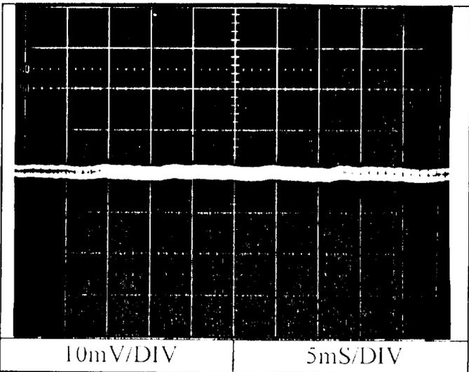
2.14 Output ripple and noise waveform
