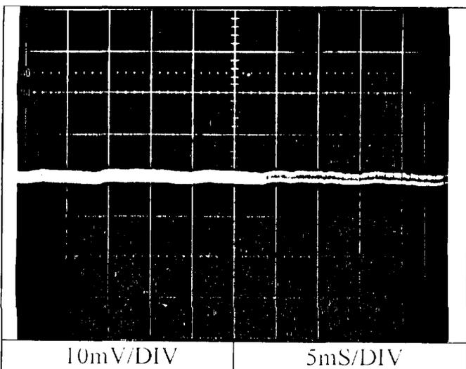
2.14 Output ripple and noise waveform
