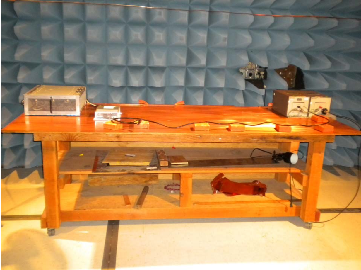
Figure D.1-1. Photo of CE102 Test Setup
