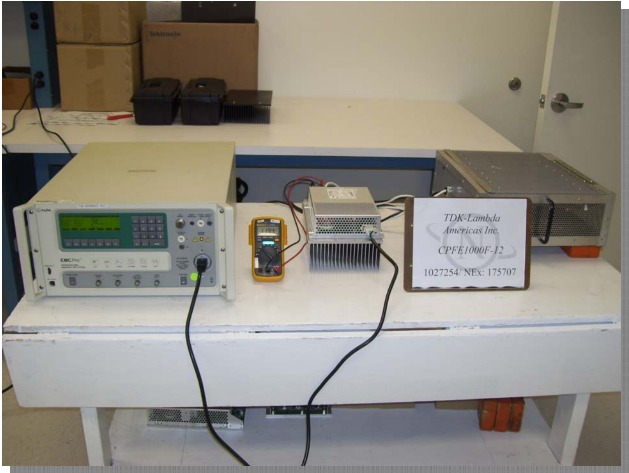
Photograph 13. Oscillatory Waves Immunity Test Configuration
