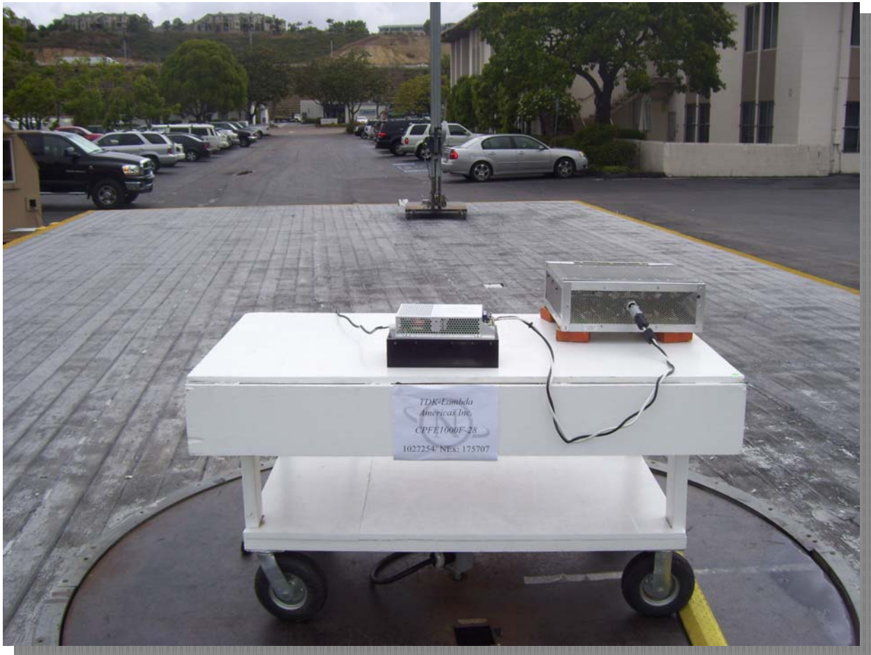
Photograph 4. Radiated Emissions Test Configuration
