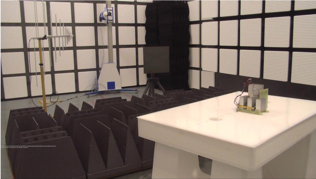
Figure 26 - Radiated Electric Field Immunity, Test Setup Photograph, Face A
