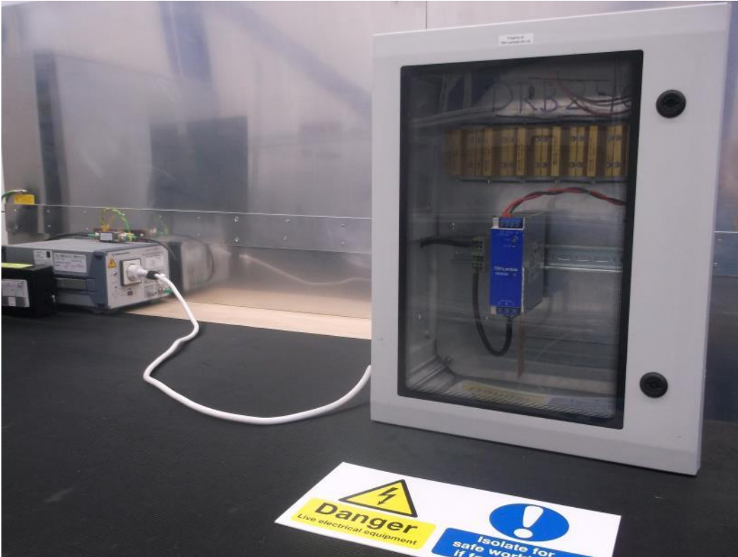
Figure 16 - Conducted Emissions Test Setup, DRB240-48-1
