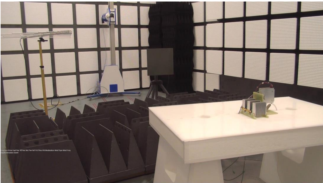
Figure 27 - Radiated Electric Field Immunity, Test Setup Photograph, Face B
