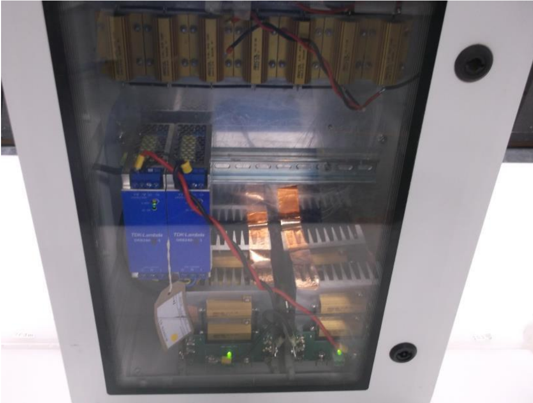
Figure 13 - Test Configuration, Radiated Emissions, In Enclosure, DRB120-48-1 x2 in series
