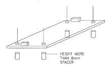
And allowable area by metal pieces is 9mm from each PCB corners. Refer to figure below.
