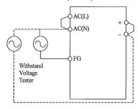
Output - FG( chassis ) 500VAC 1min. ( 100mA )
