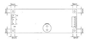
When mounting this power supply into host equipment, please leave 4mm minimum spacing between all parts of the PCB assembly except solder side and the earthed chassis of the host equipment.
