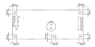
When mounting this product into host equipment, please leave 4mm minimum spacing between all parts of the PCB assembly except solder side and the earthed chassis of the host equipment.
