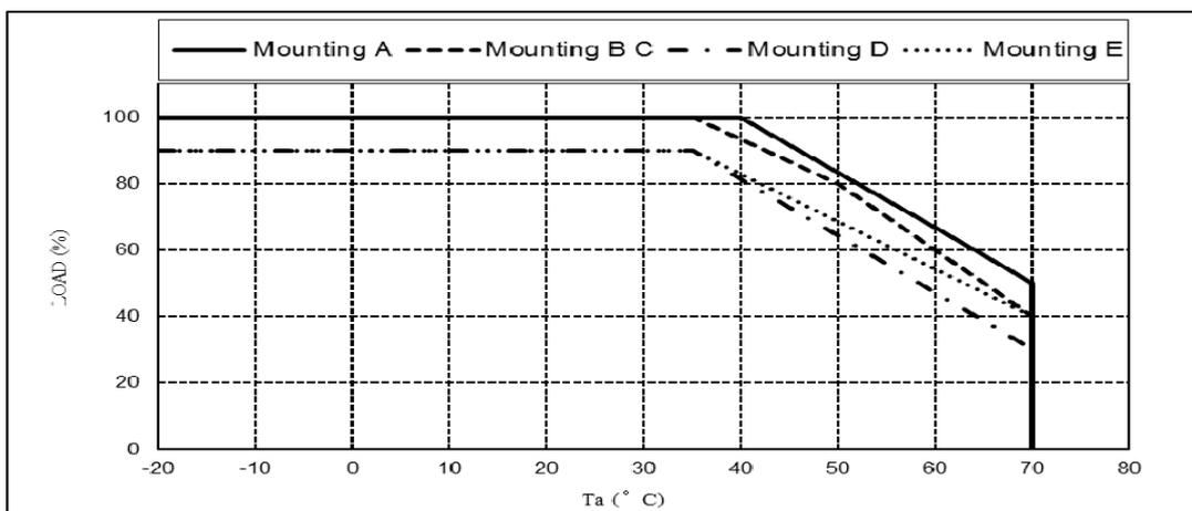
CONDITION B: Output Derating Curve for both Main Output Channel and Standby Supply.
