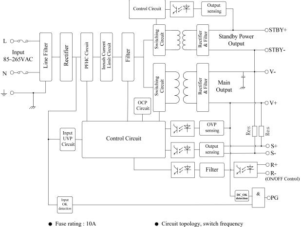
Circuit topology, switch frequency PFHC circuit: active filter 65kHz (Typ).
