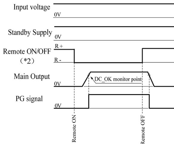
Note : (\*2) This sequence is using external voltage.
