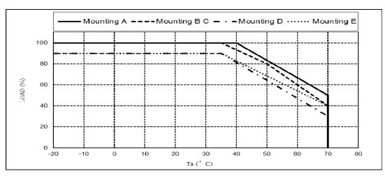
CONDITION B: Output Derating Curve for both Main Output Channel and Standby Supply. Output derating versus input voltage should be considered.
