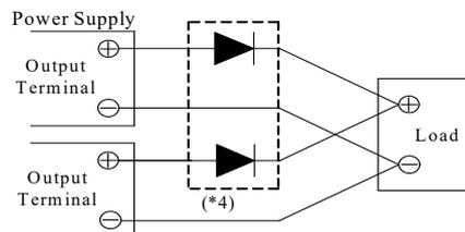
(\*4) Please select a reverse current prevention diode with maximum forward current rating more than output load current
