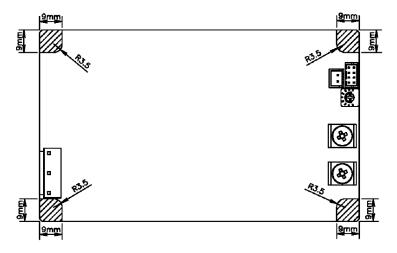
(2) Conditions to meet Isolation and Withstanding Voltage standard. Keep 5mm space from the surfaces and sides of PCB. Especially, 8mm space is necessary from the solder surface. If the space is not enough, the specification of isolation or withstanding voltage will not be satisfied.
