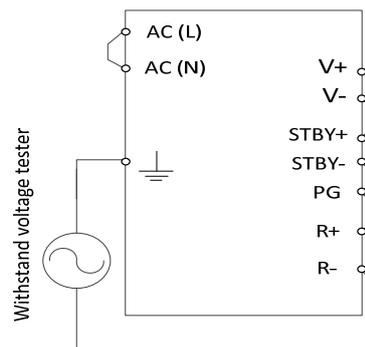
Note : In case of using external noise filter, capacitance between “Input and  $\perp$ ” might be increased. When testing withstand voltage between “Input and Output”, there is a possibility exceeding withstand voltage between “Output and  $\perp$ ” (1.5kVAC). Please check the voltage between “Output and  $\perp$ ”. If the voltage exceeding withstand voltage, please add external capacitor to “Output and  $\perp$ ”. It can decrease the voltage.
