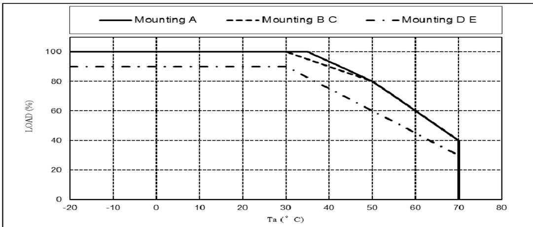
Convection cooling @ high input (176VAC~265VAC)
