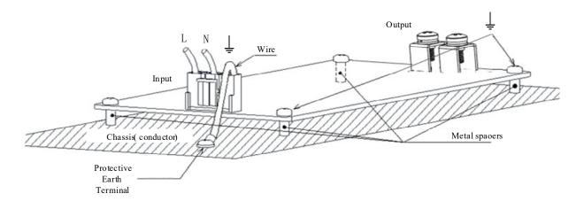
(4) For Class II end equipment,  $\stackrel{\perp}{=}$  (Functional Earth) can't be connected, All mounting holes are should be connected to the Chassis by insulated spacer. This power supply is also suitable for Class II application, however please countermeasure EMC performance before using.
