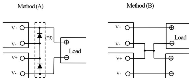
Note: In case of (A), please select a bypass diode (\*3) with maximum forward current rating more than output load current. And maximum reverse voltage must withstand each power supply output voltage.
