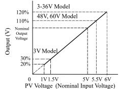
Note: Only as for the model of 3V output, the output voltage is used from 30% to 120%
