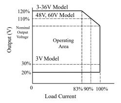
Note: Only as for the model of 48V, 60V output, the maximum output voltage is used up to 110% at 90% load current.
