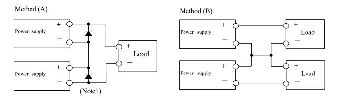
(Note1) Please connect a diode for by-pass when using method (A) of the series operation.
