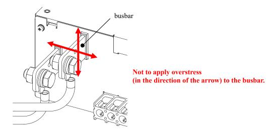
Example) Stabilize (supporting) the input/output terminals before tightening the screws.
