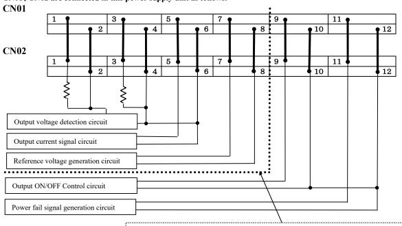
\*Output ON/OFF control circuit and the Power fail signal circuit are insulated with other circuits in the power supply. (Insulating voltage AC100V)
