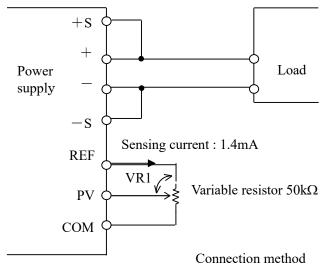
When output voltage is over rated value, please make sure that maximum output power is below rated value. Moreover, when output voltage is below rated value, please make sure that maximum output current is below rated value.
