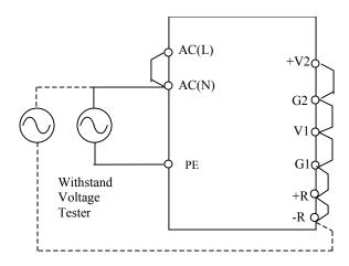
Output ~ PE (Chassis) 500VAC 1min. ( 100mA )
