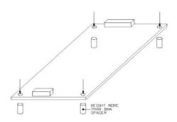
Please leave 4.5mm space from the unit surfaces and leave 4.5mm space from the sides of PCB. For the solder surface, 8mm space is necessary. If the space is not enough, the specification for insulation and withstand voltage will not be satisfied.
