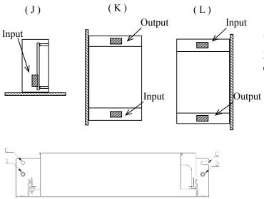
C: 1-Φ4.5 hole and R2.25 slot hole by 2-M4 screws D: Embossed tapped and countersunk holes by 2-M4 screws.
