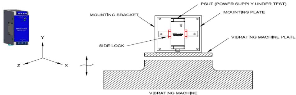
Fix the PSUT on the mounting rail with stopper on each corner.
