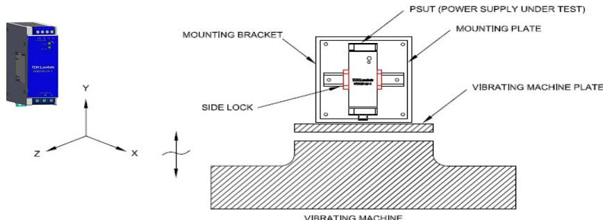
Fix the PSUT on the mounting rail with stopper on each corner.
