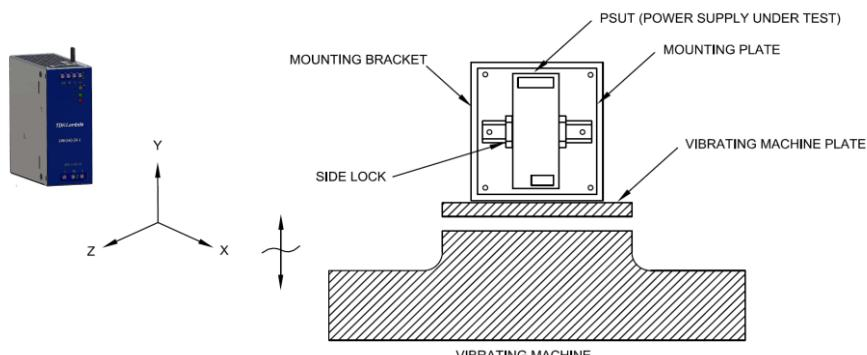
Fix the PSUT on the mounting rail with stopper on each corner.
