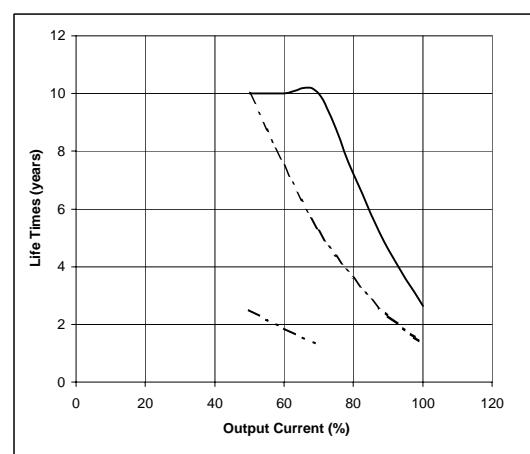
Note : E-cap life calculation is based on 8hrs/day operation.
