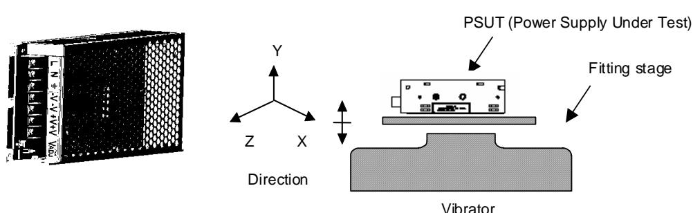
Fix the PSUT on the universal plate via two M3 tapped holes on the chassis of the power supply.
