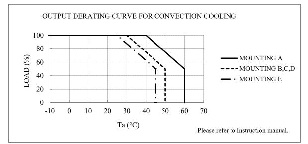
\* Load (%) is percent of total allowable output power or each maximum output current, whichever is greater.
