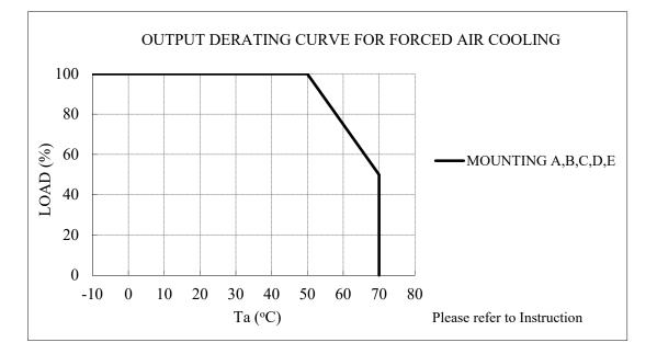
\* Load (%) is percent of total allowable output power or each maximum output current, whichever is greater.
