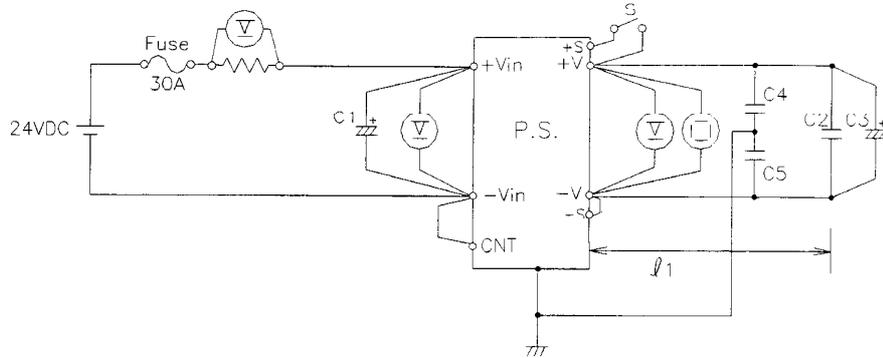
C1: 220uF Electrolytic Capacitor x 2para C3: 12V-470uF Electrolytic Capacitor  $l_1$ : 50mm
