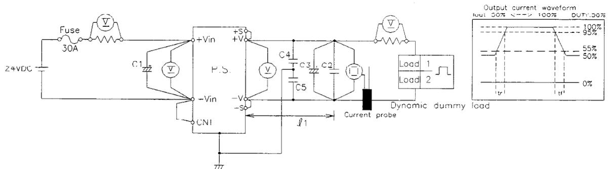
C1: 220uF Electrolytic Capacitor x 2para C3: 12V-470uF Electrolytic Capacitor I1: 50mm
