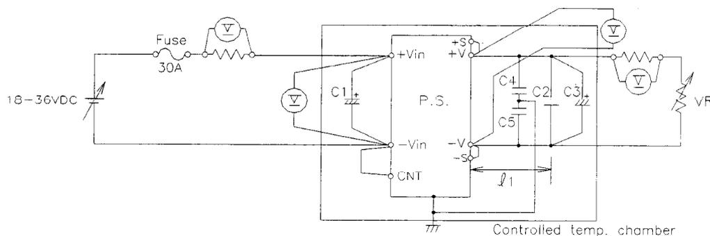
C1: 220uF Electrolytic Capacitor x 2para C3: 12V-470uF Electrolytic Capacitor  $l_1$ : 50mm
