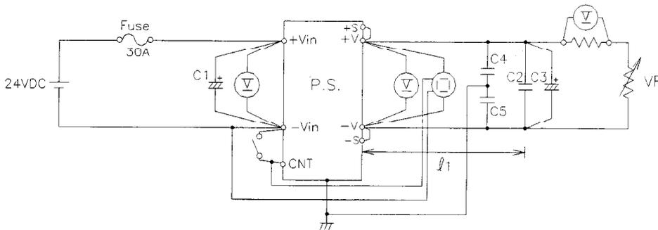
C1: 220uF Electrolytic Capacitor x 2para C3: 12V-470uF Electrolytic Capacitor I1: 50mm
