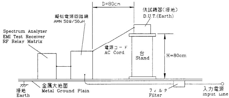
(b) 雑音電界強度 (輻射ノイズ) Radiated Emission Noise
