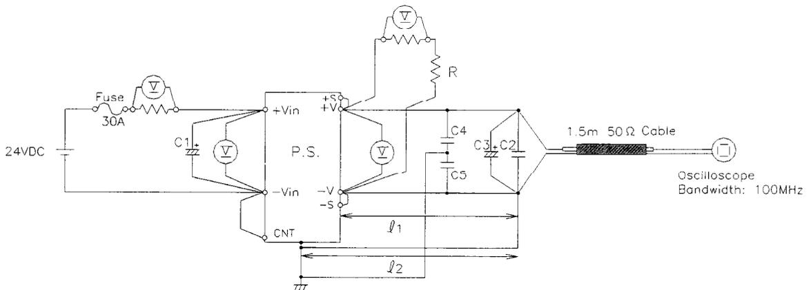
C1: 220uF Electrolytic Capacitor x 2para C3: 12V 470uF Electrolytic Capacitor  $l_1, l_2$ : 50mm
