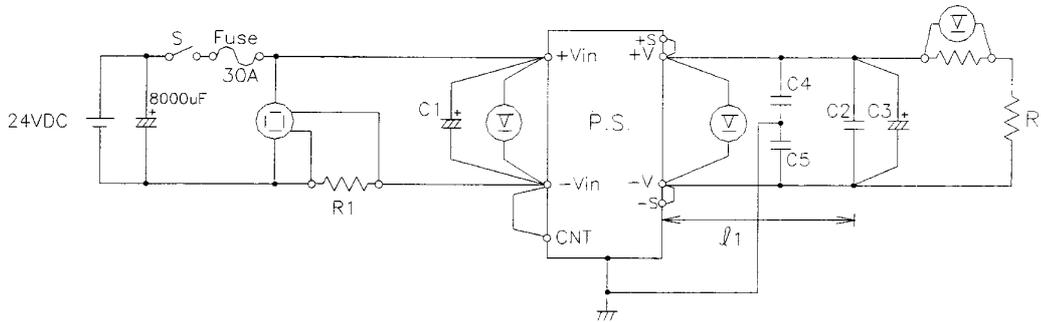
C1: 220uF Electrolytic Capacitor x 2para C3: 12V-470uF Electrolytic Capacitor R1: 0.01Ω
