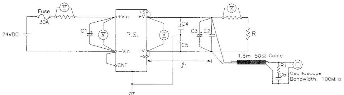
C1: 220uF Electrolytic Capacitor x 2para C3: 12V-470uF Electrolytic Capacitor C6: 4700pF Ceramic Capacitor
