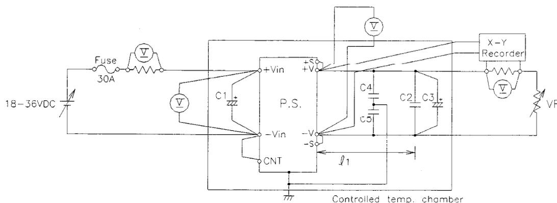
C1: 220uF Electrolytic Capacitor x 2para C3: 12V-470uF Electrolytic Capacitor  $l_1$ : 50mm
