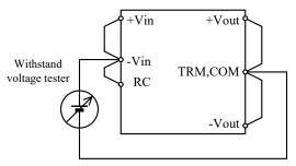
Fig.6-12 Withstand Voltage Test for Input - Output
