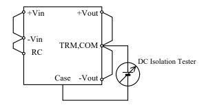
Fig.6-15 Isolation Resistance Test
