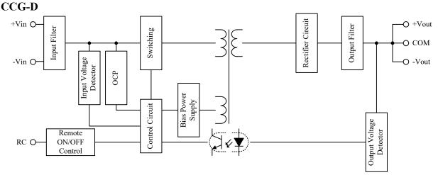
Switching Frequency(fixed): 430kHz
