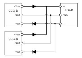
Fig.6-8 Redundant Operation Connection (CCG-D)
