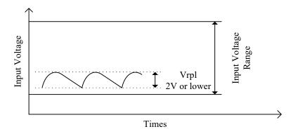
Fig.6-1 Input Ripple Voltage
