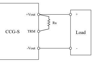
Fig.6-2 Basic Connection for Output Voltage Trim Down
