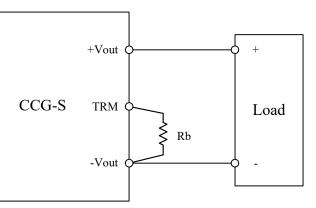
Fig.6-3 Basic Connection for Output Voltage Trim Up
