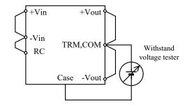
Fig.6-13 Withstand Voltage Test for Input - Case
