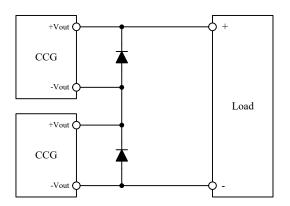
Fig.6-9 Series Operation for High Output Voltage
