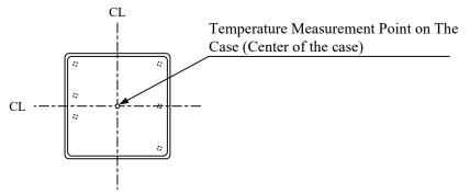
Fig.7-3 Temperature Measurement Point on The Case
