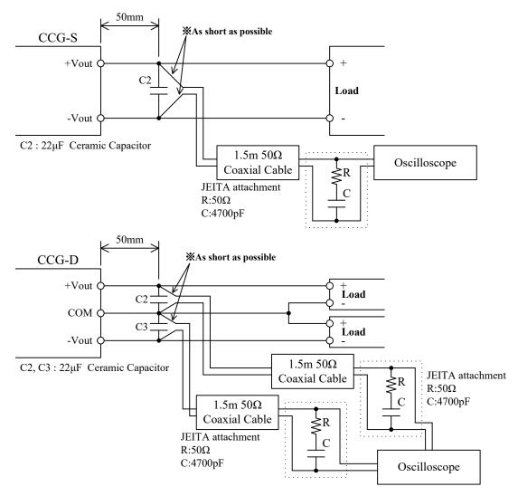
Fig.6-4 Measurement of Maximum Output Ripple and Noise
