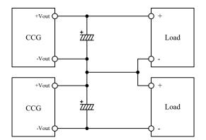
Fig.6-10 ±Output Series Operation
