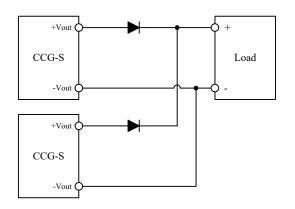
Fig.6-7 Redundant Operation Connection (CCG-S)
