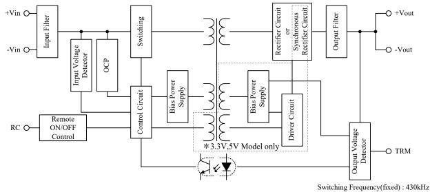
**CCG30-S** Rectifier Circuit Rectifier Circuit +Vin O -O +Vout Synchronous Output Filter Input Filter Switching  $\stackrel{\scriptstyle \checkmark}{}$  $\mathbf{or}$ Input Voltage Detector -Vin C O -Vout OCP Bias Power Supply **Bias** Power Supply Control Circuit Driver Circuit Remote RC O ON/OFF Output Voltage Detector Control ₩3.3V,5V Model only -O TRM
