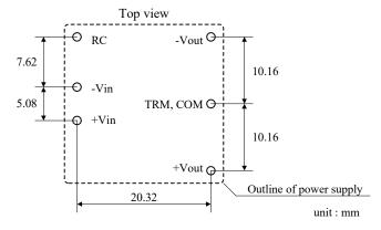
Fig.8-1 Dimension of Mounting Hole Position
