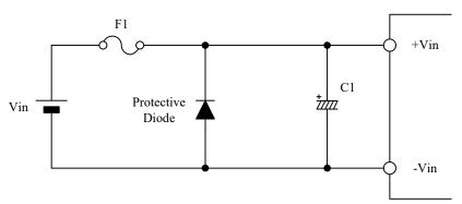
Fig.5-2 Protection for Reversed Input Connection
