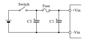
Fig.1-3 Input Filter with Input Switch
