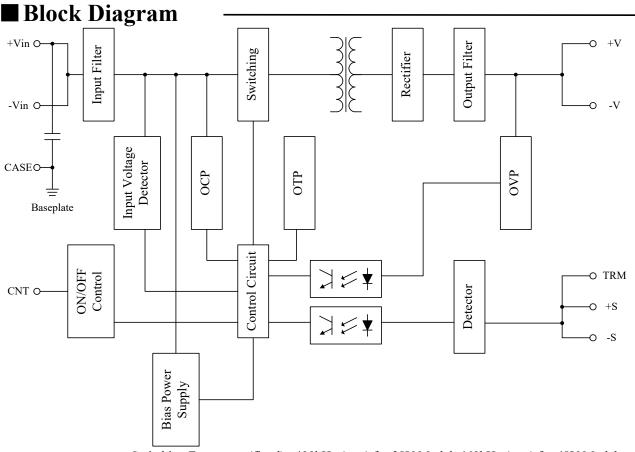
Switching Frequency (fixed) : 400kHz (typ.) for 28V Model, 460kHz (typ.) for 48V Model
