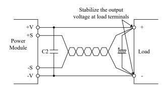
Fig.9-1 Remote Sensing is in Use
