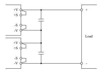
Fig.12-1 Series Operation due to High Output Voltage
