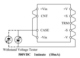
Fig.19-2 Withstand Voltage Test for Output-Baseplate
