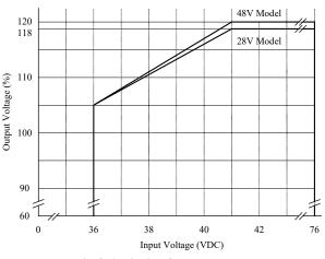
Fig.2-1 Limit of Input Voltage
