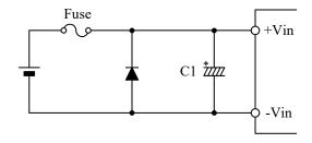
Fig.1-5 Protection for Reversed Connection of Input
