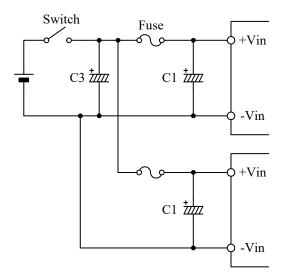
Fig.1-4 Input Filter when Plural Power Modules
