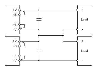
Fig.12-2 Series Operation due to ±Output
