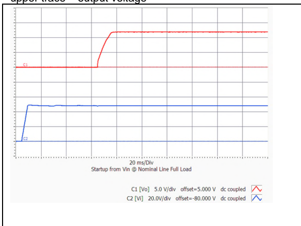
iQE4W011A120V-001 Typical startup characteristic from input voltage application at full load. Upper trace - output voltage, lower trace –input voltage
