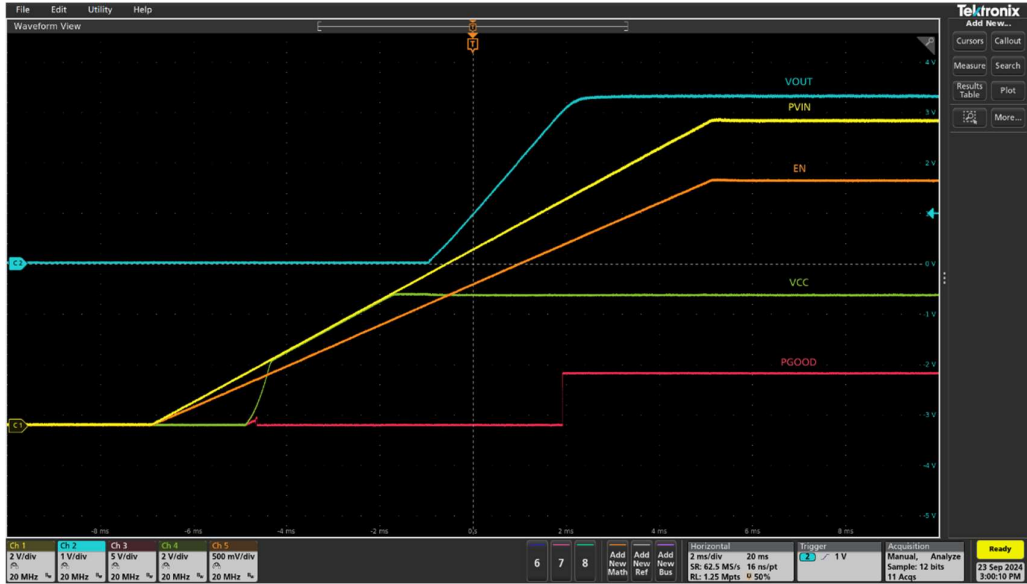
Figure 3 Startup with no load (Ch1 : PV_{IN} , Ch2: V_{OUT} , Ch3: PG, Ch4: V_{CC} , Ch5: Enable)
