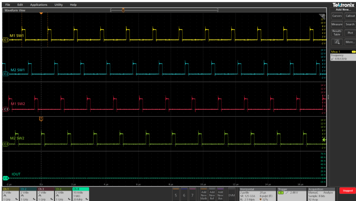
Figure 13 Switch node waveforms at no load
