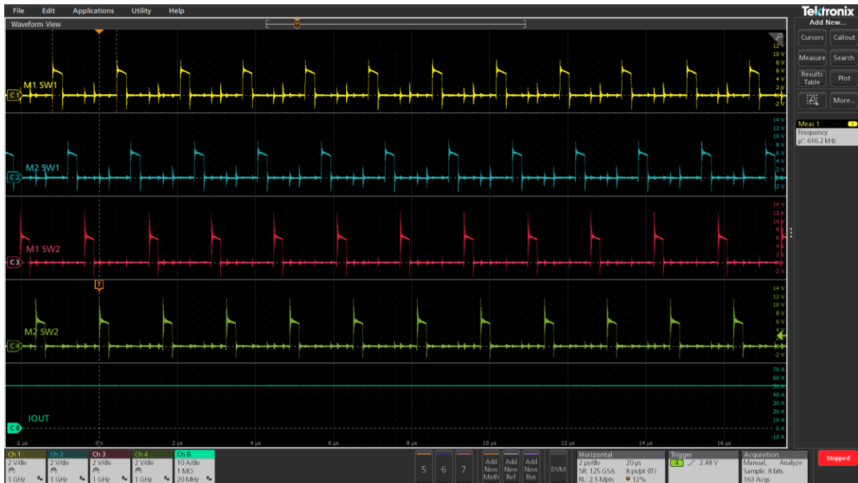
Figure 14 Switch node waveforms at 50A
